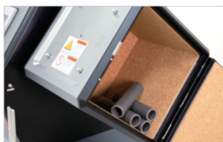
Pilling box inside
